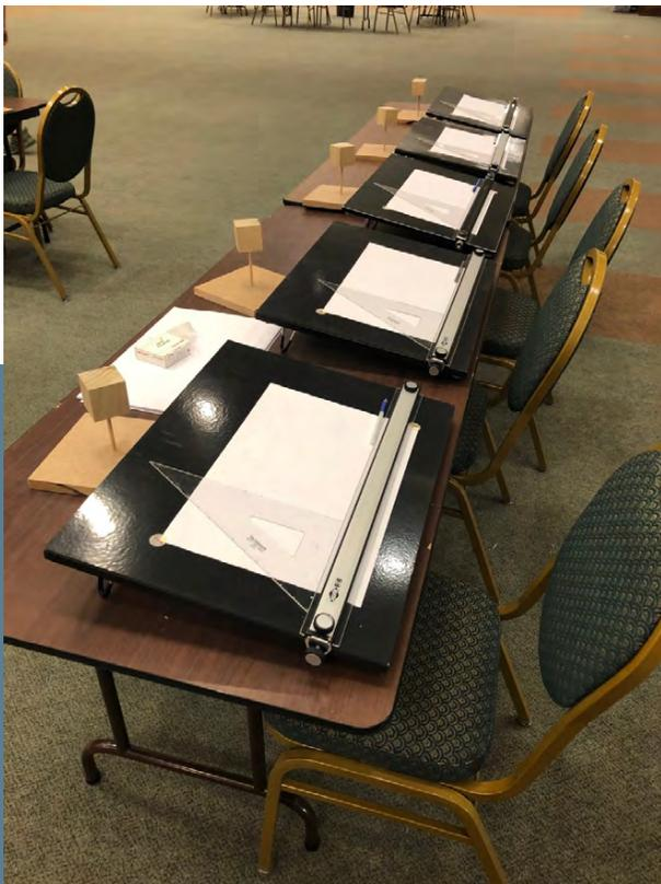
Figure 1. Tactile Drawing Board
