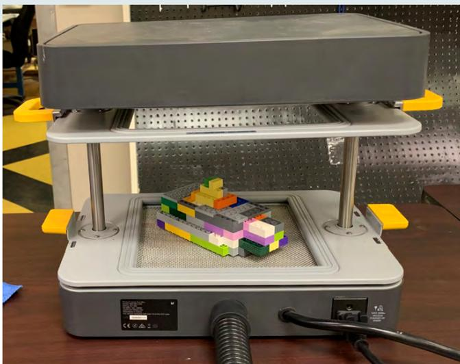
**Figure 1.** Thermoform Machine with Sample Boat Mold
