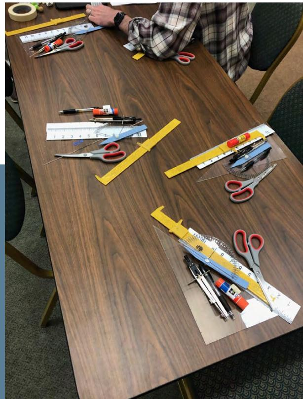
Figure 2. Manual Tactile Drawing Tools
