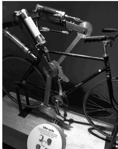
Figure 6. Bike Cycle exhibit which challenges visitors to coordinate timing and sequence of robotic legs to spin a bicycle wheel.
