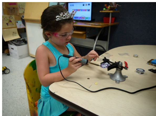
A student practices her soldering skills to make a button with an LED light.
